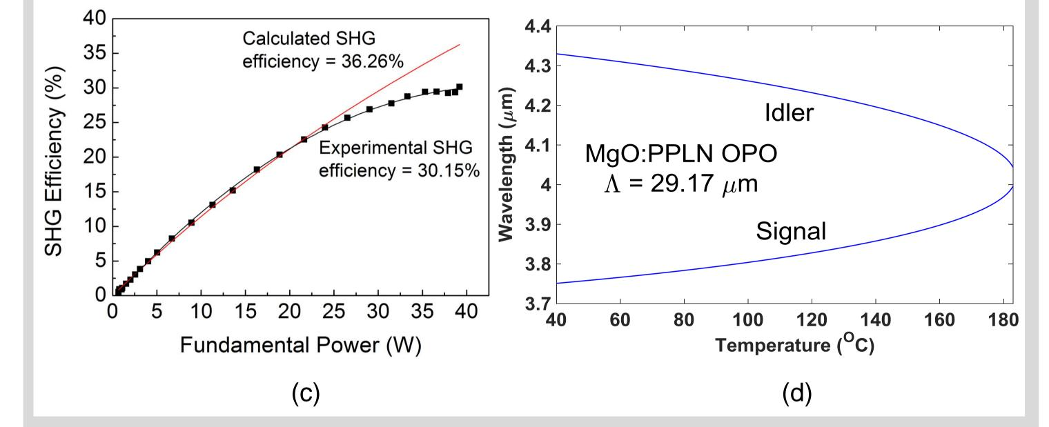
(c) Theoretically calculated and experimentally obtained SHG conversion efficiency vs fundamental power. (d) Temperature tuning curve of MgO:PPLN OPO with grating period 29.17  $\mu$ m. Specific applications of 1.005 µm source: 1. In the study of energy dynamics of light-harvesting proteinpigment complexes [1] 2. In the study of photovoltaics structure [2]
