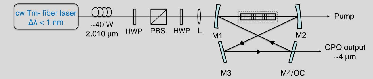
Mirrors M1 and M2: r =150 mm; highly reflecting for signal and idler for 4 µm (doubly resonant operation), highly transmitting for pump. M3: plane mirror, M4: plane output coupler. For OPO, L:  $f = 100 \text{ mm}, w_0 \sim 80.6 \mu \text{m},$  $\Lambda$  = 29.17 μm, ξ =1.16, cavity length = 898 mm.
