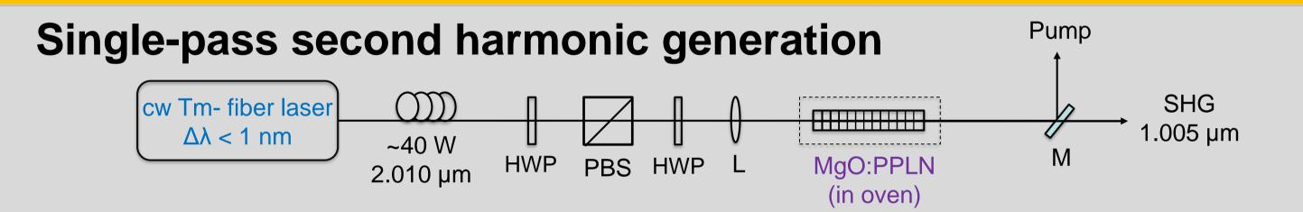
The fundamental beam is focused to a measured beam waist radius  $w_0 \sim$ 51.5  $\mu$ m at the center of 50-mm-long crystal with grating period  $\Lambda = 30$  $\mu$ m (focusing parameter  $\xi$  = 2.84) using lens L: f =150 mm. HWP = half-wave plate, PBS: polarising beam splitter, M: dichroic mirror.
