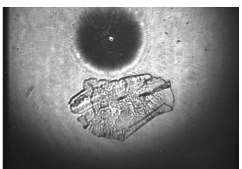
Acquired upconverted transmission image of a human esophagus sample at  $4\mu$ m. Images can be acquired in real time at a rate of 22 images per second.
