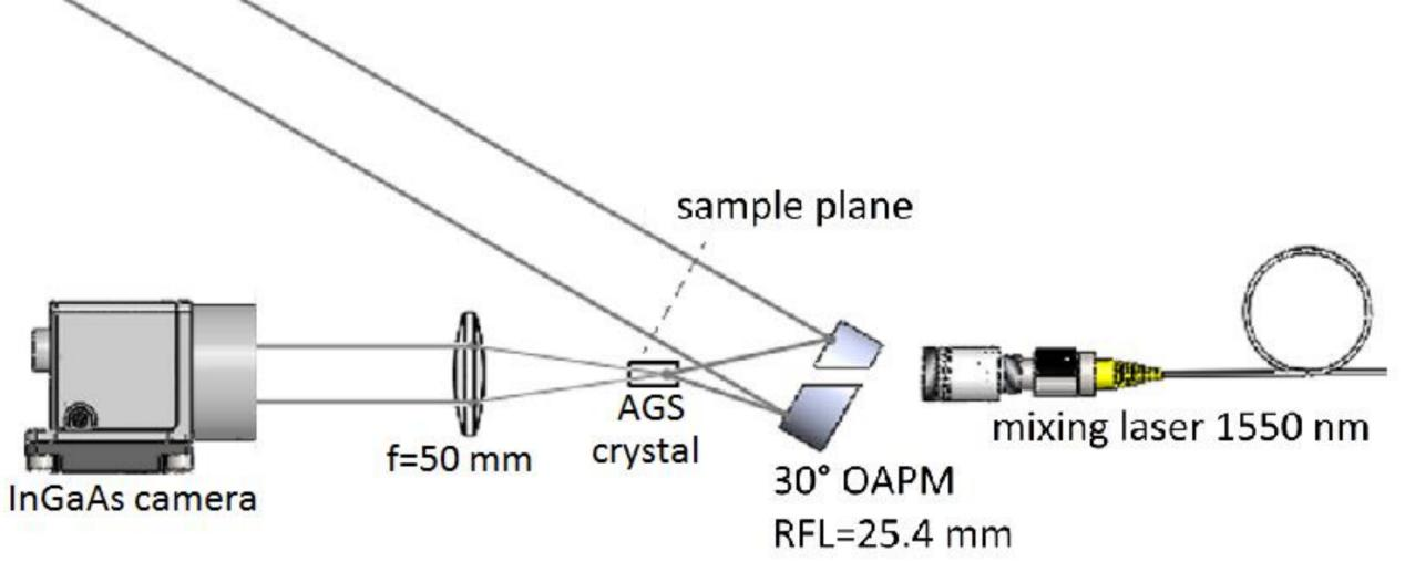
Top view schematic representation of the pulsed upconversion imaging setup. The use of OAPMs make for a mostly achromatic setup. The broadband signal pulse is combined with the 1550 nm pump pulse through a hole drilled through the OAPM.
