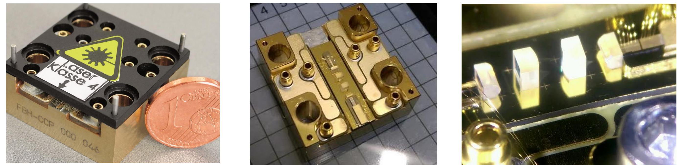
Fig. 1 Images of the developed 4 nm tunable hybrid MOPA laser, including the micro-lenses used for the optical coupling. Left image ©FBH/schurian.com
