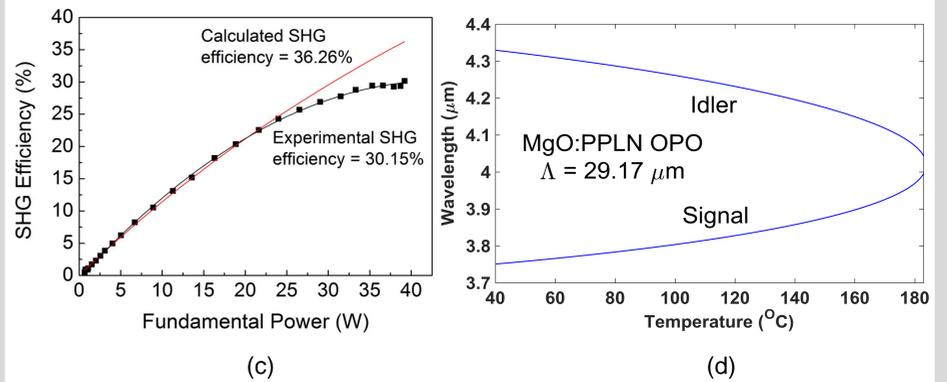
(c) Theoretically calculated and experimentally obtained SHG conversion efficiency vs fundamental power.
