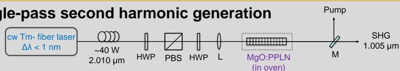
The fundamental beam is focused to a measured beam waist radius  $w_0 \sim 51.5 \mu\text{m}$  at the center of 50-mm-long crystal with grating period  $\Lambda = 30 \mu\text{m}$  (focusing parameter  $\xi = 2.84$ ) using lens L:  $f = 150 \text{ mm}$ . HWP = half-wave plate, PBS: polarising beam splitter, M: dichroic mirror.
