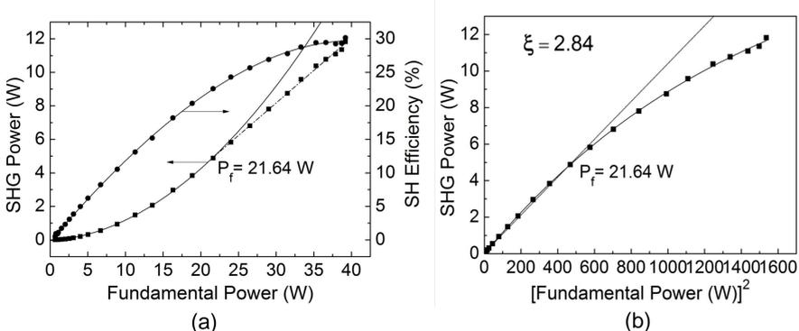
(a) Dependence of measured SHG power and corresponding conversion efficiency on the incident fundamental power
