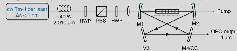
Mirrors M1 and M2:  $r = 150 \text{ mm}$ ; highly reflecting for signal and idler for 4  $\mu\text{m}$  (doubly resonant operation), highly transmitting for pump. M3: plane mirror, M4: plane output coupler. For OPO, L:  $f = 100 \text{ mm}$ ,  $w_0 \sim 80.6 \mu\text{m}$ ,  $\Lambda = 29.17 \mu\text{m}$ ,  $\xi = 1.16$ , cavity length = 898 mm.
