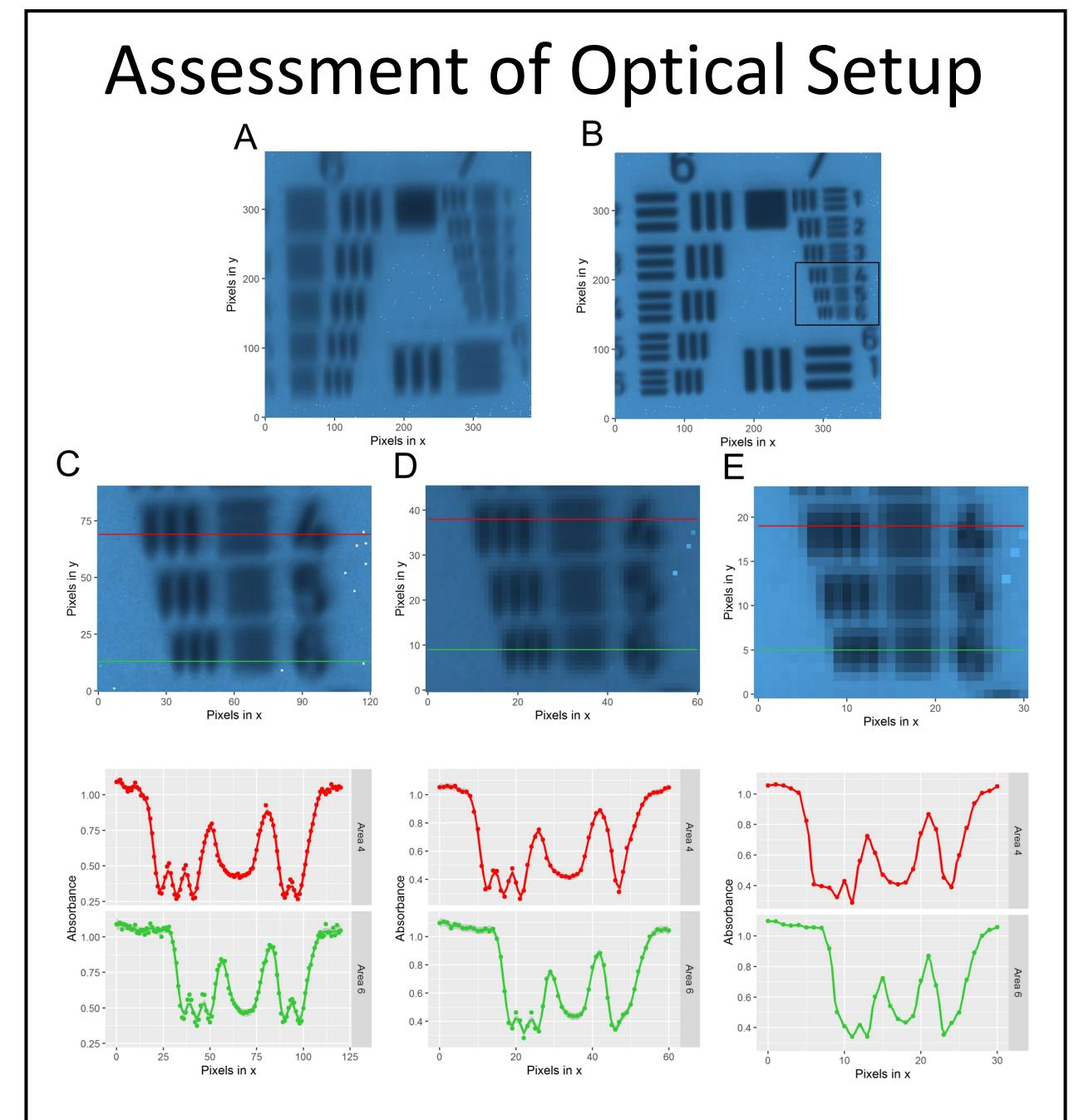
FTIR image of chrome on glass USAF 1951 target. Average intensity per pixel in the region 1400–1000 cm<sup>-1</sup> (A) and 3900–3800 cm<sup>-1</sup> (B); zoomed in area of the boxed region from B with its corresponding average intensity along the coloured lines (C); 2×2 (D) and 4×4 (E) binned image of B with its corresponding average intensity along the coloured lines. Published in Vibrational Spectroscopy from *Nallala et. al.* [1].
